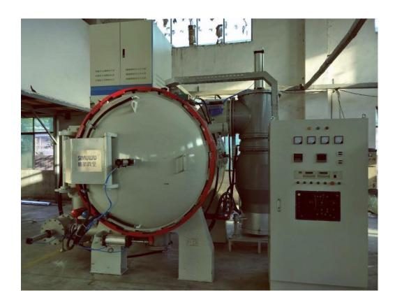
This vacuum furnace applies to stainless steel, tungsten, molybdenum and W-Mo alloy materials or debinding and sintering process.
