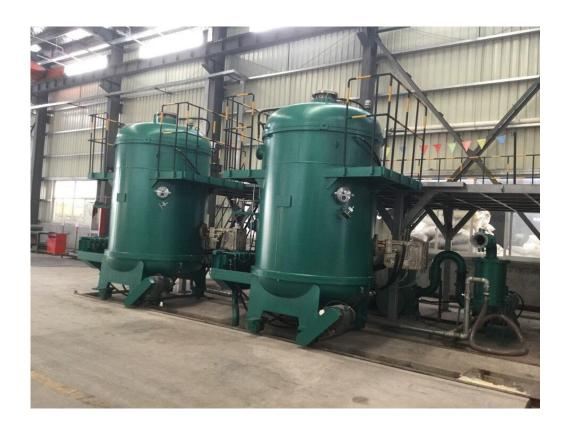
This equipment mainly usage is doing powder hot press forming process under vacuum (or inert gas atmosphere), high temperature condition, make high quality big size base composite shielding material, it use vacuum induction hot pressing process.
